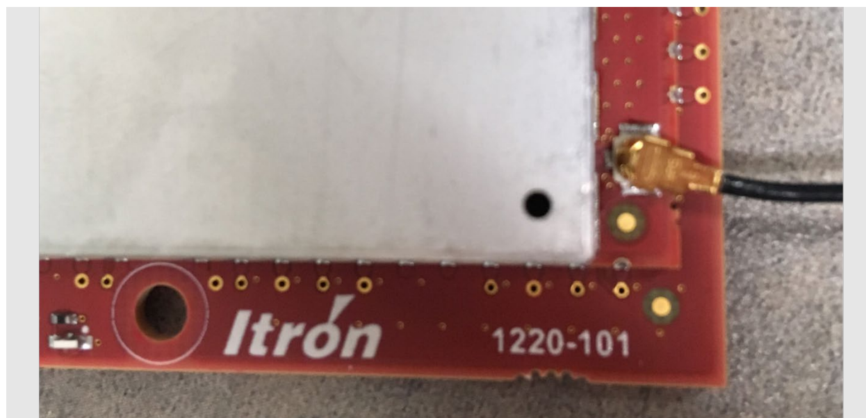
Figure 11: Antenna cable attached to uFL connector
